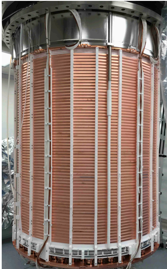
TPC (5.9 t LXe, 4 t fiducial), 1.3 m diameter, 1.5 m tall
