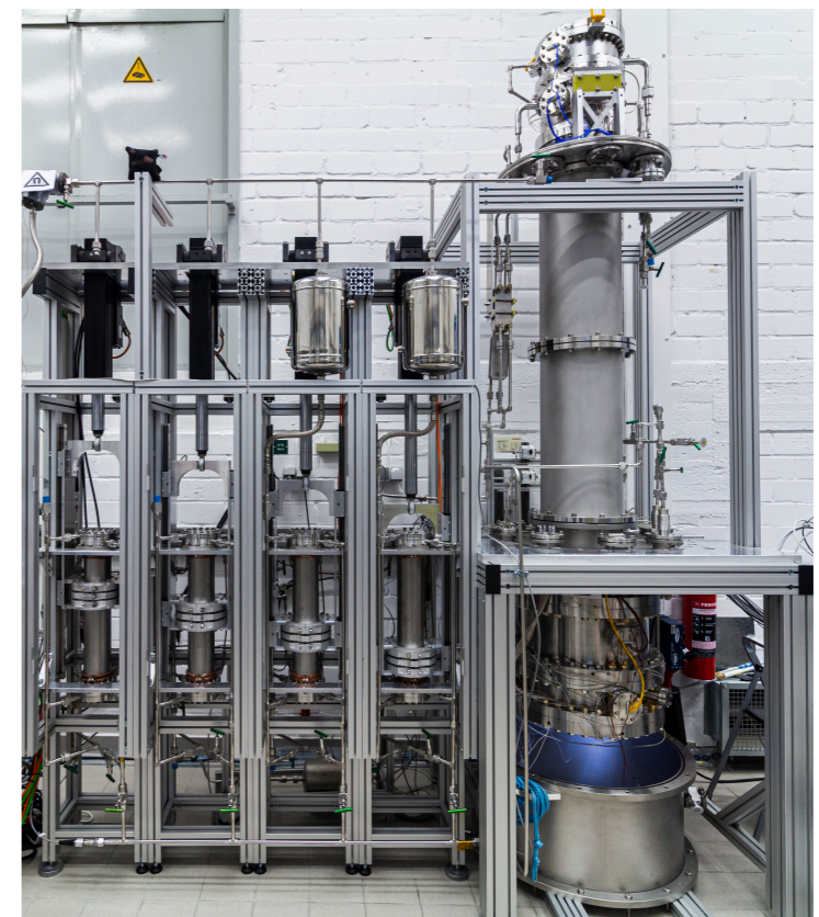
Rn distillation column (reduce ^{222}Rn - hence also ^{214}Bi - from pipes, cables, cryogenic system)
