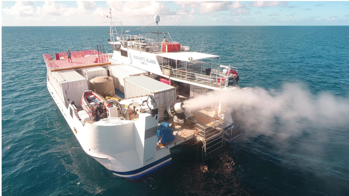
During a field trial, a turbine generates plumes of seawater droplets that rise into the sky. Credit: Brendan Kelaher/SCU
